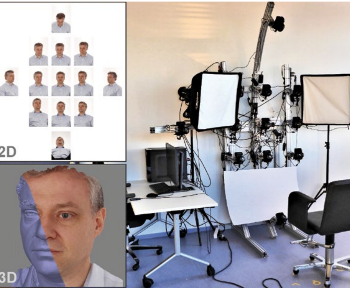
The K13 recording stand for facial biometrics consists of 13 cameras that capture images simultaneously
