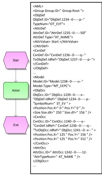
Fig. 4 Representation of an EPC with AML
