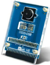
Figure 4.6: Five megapixel CCD camera D5M from Terasic Technologies.
