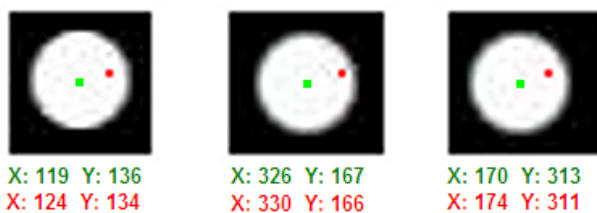
Figure 4.4: Detection of a centre point of a round-shaped BLOB showed a systematic error in the X and the Y axes.
