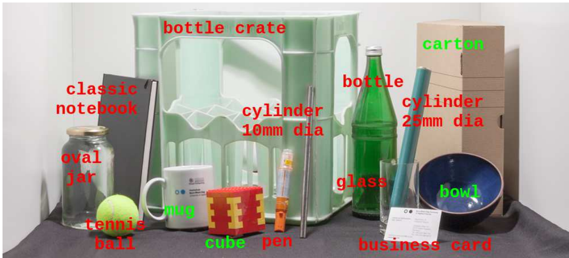
Figure 3.11: Objects used for grasping: classic notebook, oval jar, tennis ball, mug, cube, bottle crate, small cylinder, pen, bottle, glass, business card, bowl, cylinder large, carton ( 7.6 \times 26 \times 37.5 \text{ cm}^3 ). Only objects in red were used in controlled transport.
