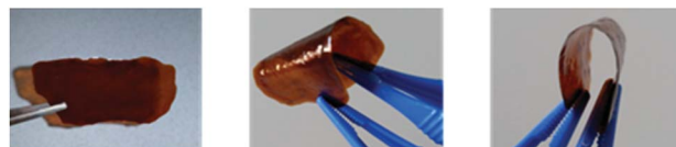
Fig. 20 Flexible lignin-PU coatings of different color intensity according to the lignin content up to 70% synthesized with KL isolated at pH 4.
