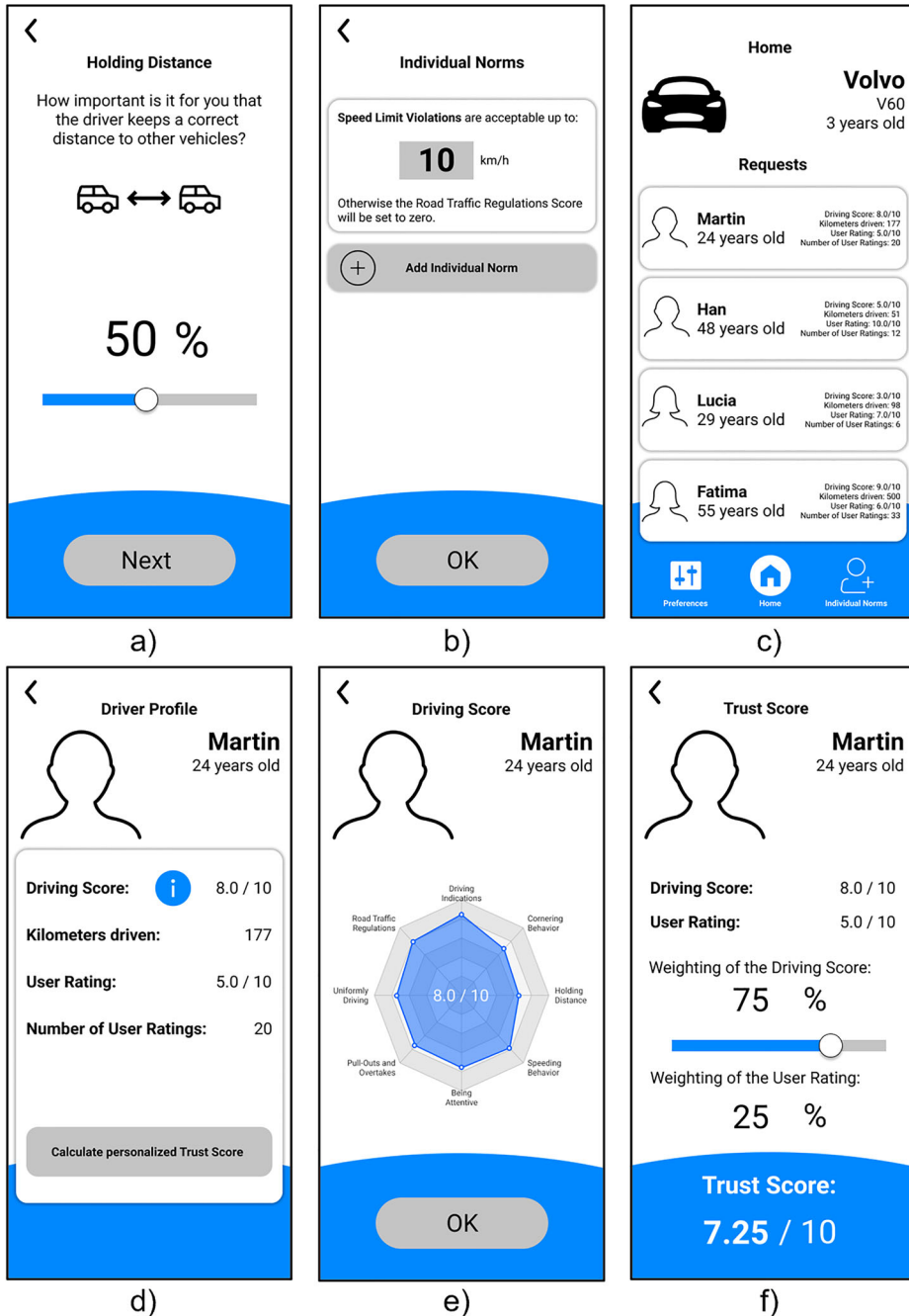
Figure 2. Clickable Prototype – a) exemplary preference weighting, b) individual norm settings, c) home screen with requests, d) exemplary driver profile, e) exemplary Driving Score drill-down, f) exemplary Trust Score weighting
