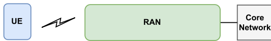
FIGURE 1. A simple overview about the basic components of a mobile network. This overview will be further specified in the following.
