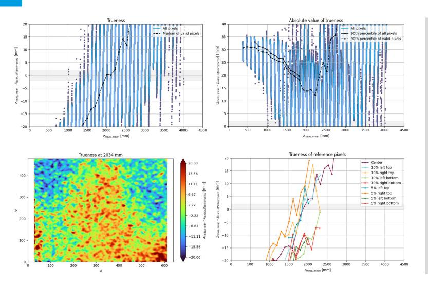
**Trueness:** Closeness between average of a large series of test results and its accepted reference value (ISO 5725-1:1994). Here the difference between the average of 100 frames and the laser distance sensor's measured value is determined.
