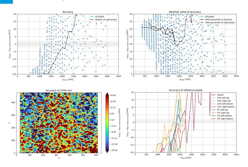
Accuracy: Closeness between a single test results and its accepted reference value (ISO 5725-1:1994). Here the difference between each pixel's distance value and the laser distance sensor's measured value is used. In contrast to the trueness, the pixel's values are not averaged. Due to this the accuracy represents a combination of systematic and statistic errors.
