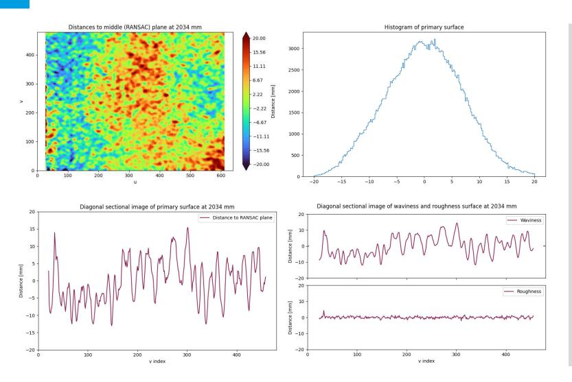
**Primary surface:** Surface after removing the form surface. Here a plane derived with the RANSAC algorithm. (ISO 21920-2:2021)
